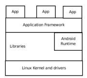
Figure 1.5: Android software stack
