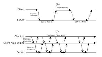
Figure 1.6: Workflow comparison between (a) classic HTTP clients and (b) AJAX clients
